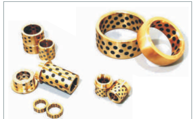
Graphite impregnated bushes providing self lubrication, increased toggle mechanism life & clean molding operation.
