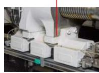
Close loop Tie Bar position feedback with precise magnetic transducer
